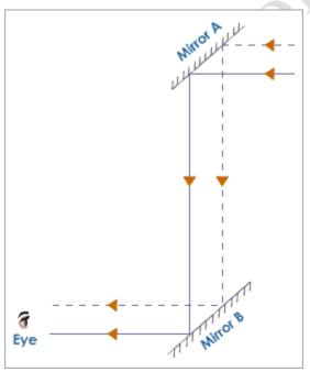
The angle of incidence is equal to 45° which exceed the critical angle for glass and therefore total internal reflection occurs.
