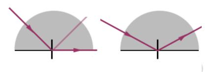
The angle of incidence is equal to the critical angle.
