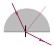
The angle of incidence is less than the critical angle.
