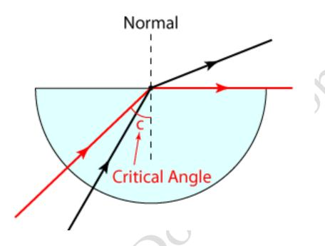
The experiment is set up as shown above in a darkened room. The ray of light that is emitted from the ray box is directed to the centre of the curvature of the semicircle glass block.
