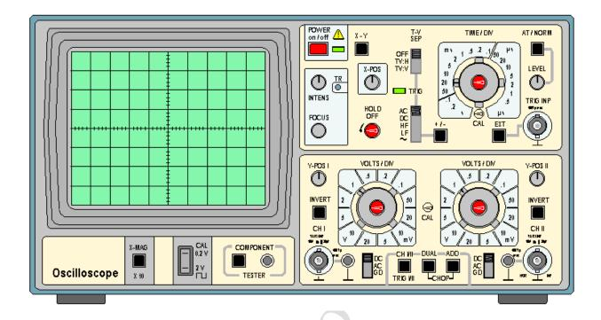
Cathode Ray Oscilloscope (CRO) uses a cathode ray tube to produce visible graphical representations of electrical signals.
