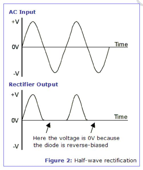
Half wave rectification of alternating current produces a flow of current that exists in only one direction. Therefore half wave rectification of alternating current produces direct current.
