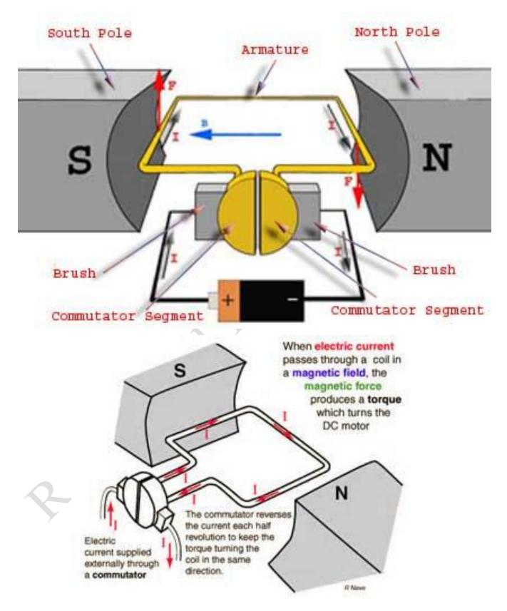
The D.C. Motor consists of a coil of wires found between opposite poles of a permanent magnet. From the coil there are two wires which lead to the split commutator. The commutator is connected to the rest of the circuit via spring contacts. These spring contacts allows the split ring commutator to rotate without the opening the circuit.
