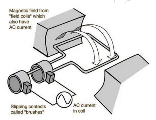
The a.c. generator produces alternating current when supplied with motion. It consists of a wire coil placed between the end of a magnet. When the coil rotates an electric current is generated. The wires of the coil cuts the magnetic field lines and this results in the formation of an induced current.
