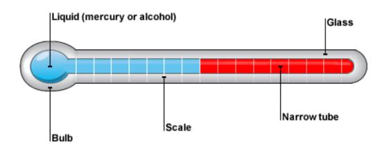
The above diagram shows a liquid-in-glass thermometer. The liquid may either be mercury or alcohol.
