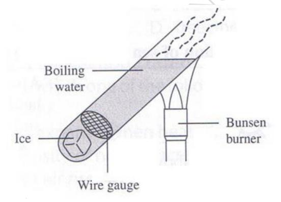
The boiling tube is set up as shown above. On heating the top layer of the water, without the ice melting completely. The metal gauze is used to prevent the ice from floating.
