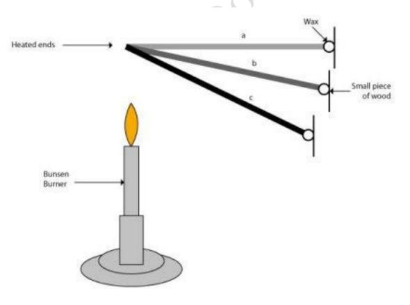
The experiment is set up as shown in the diagram using identical size metal rods and wax droplets. The time taken for the wax droplet to fall will give an indication as to the conduction of the metals.
